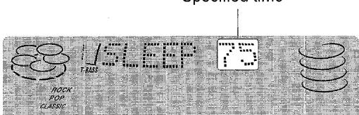
**To check the time remaining until the power is turned off**
